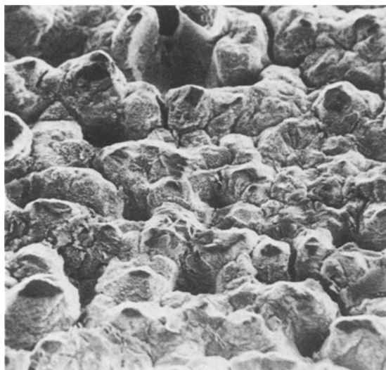
Fig. 2. SEM photomicrograph ( \times 960 ) showing the block morphology obtained with the addition of 40 \text{ mg dm}^{-3} Gum Tragacanth.
